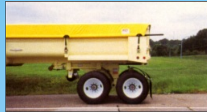
After locking the tandem, the trailer can be dumped as any other end dump.
