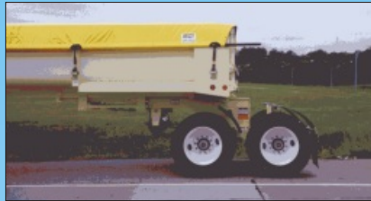
In its running configuration, the "Bridger" extends the internal and external bridges and thus increases the payload.
