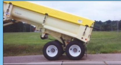
To dump the load over the rear tandem, the trailer brakes are set and the trailer is moved back to the proper dumping position.
